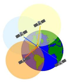
This way we can obtain the distance between each satellite and the receiver. The distance is equal to the radius of the sphere.
