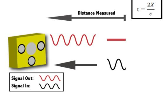
The above picture shows a more realistic implementation of the time of flight principle. A light source (yellow box) emits a light pulse which reflects on the black object. A clock starts counting time from the moment of the emission and on. The light reflects and goes back to the yellow box where it is detected. Its arrival time is recorded.
